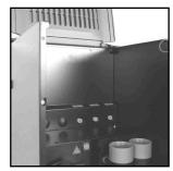
5. Empty contents of canisters and place back into machine. Make sure to place lids on canisters. (Rinse with water to clean, if desired)
