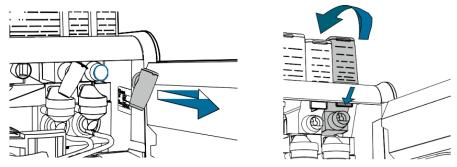
5. Empty contents of canisters and place back into machine. Make sure to place lids on canisters. (Rinse with water to clean, if desired)
